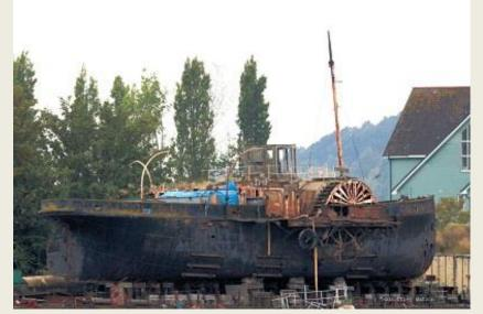
finished the work by using materials that were already available in the yard. As a result some aspects of the vessel were better than the original specification. Unfortunately other components turned out to be unsuitable. It was soon discovered that the boilers they used could not supply enough steam for the large diagonal compound engines. A maximum of only 11 knots was achieved instead of the
