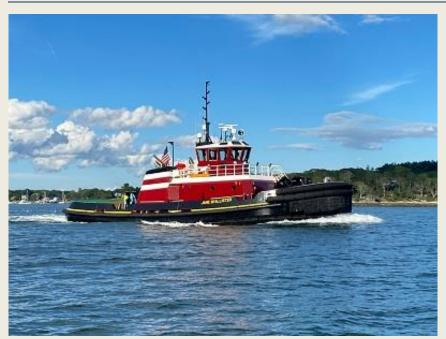
McAllister Towing is proud to announce the arrival of the tug Jane McAllister. The Jane is equipped with 3516E Tier IV Caterpillar engines powering twin Schottel SRP 490 Zdrive units. Packed into her 93' x 38' hull 6,770 producing horsepower, the JANE achieved over 91 short tons during her ABS bollard pull certification. Combining her eco-friendly CAT engines with Markey winches on the bow and stern makes the lane one of the most
