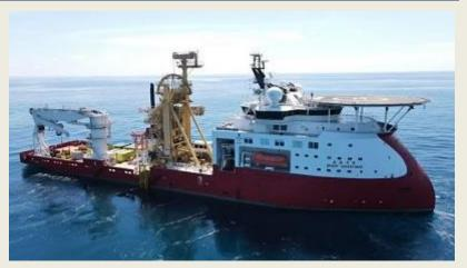
wind developments. Huisman has adapted the carousel design, which is based on proven carousel and storage components, to maximize use to the vessel's hold capacity for cable-laying or pipelaying. Delivery is scheduled for the first half of 2024. The optional cable-lay system is a new concept designed for temporary installation on, for example, a multi-purpose offshore vessel that could be quickly mobilized or demobilized. *(Source: Offshore)*
