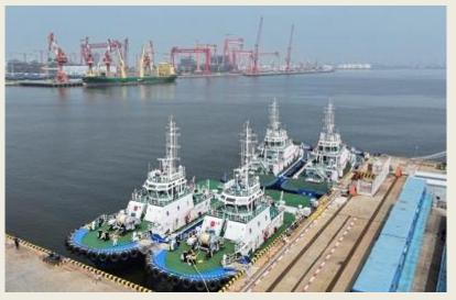
A "green fleet" consisting of four fully electric-powered harbour tugboats set sail from a port in north China's Tianjin Wednesday. These four tugboats form the largest fleet of their kind in northern China, which will primarily assist various vessels with port entry, exit, docking, and undocking within Tianjin Port waters. Unlike conventional tugboats, the electric ones operate with zero exhaust emissions and low noise. Each of them boasts
