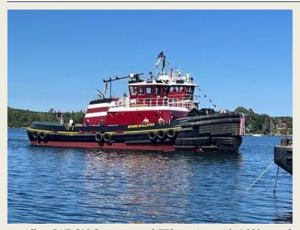
Washburn & Doughty Associates Boothbay, Inc., Maine, has launched a new for Mcallister tractor tug Towing and Transportation Co. Inc., New York. The 93'x38' Gerard McAllister offers 6,770 hp and a bollard pull of 84 tons. It features a pair of EPA Tier 4compliant Caterpillar engines that power Schottel SRP 490 FP Z-drive units. The tug is equipped with 99-kW John Deere 4045 AFM85 EPA Tier 3 generators, Markey Machine winches on the bow and stern,
