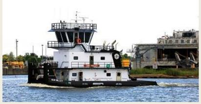
Valley measures 67 feet, 6 inches by 28 feet, with a depth of 9 feet, 6 inches and a design draft of 7 feet, 9 inches. The pilothouse provides an eye level of 29 feet, 10 inches. The Sun Valley gets its 1,600 hp. from a pair of Mitsubishi S6R2 Tier 3 diesel engines supplied by Laborde Products. On
