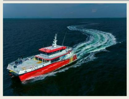
A new crew transfer vessel (CTV), designed by naval architect Chartwell Marine, has been delivered to Singaporebased offshore vessel operator Pacific Radiance. The vessel, named **Prosperous 6**, has already completed sea trials, achieving over 25 knots at 85 per cent engine load. During a bollard push test, the CTV delivered over 17 tonnes of bollard push, according to Chartwell Marine. When operating at 20 knots, **Prosperous 6** used approximately 20 per cent less fuel than
