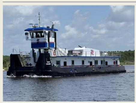
Steiner Shipyard, Bayou La Batre, Ala., has delivered the 94'x34'x12' retractable pilothouse towboat Gage Golding to Golding Barge Line Inc., Vicksburg, Miss. The new towboat is an addition to the Golding fleet, not a replacement. Designed by the shipyard Marine, and Sterling Fairhope, Ala., Gage Golding is powered by a pair of Tier 4 Caterpillar 3512 diesel engines from Pucket Machinery, Gulfport, Miss. The Cats
