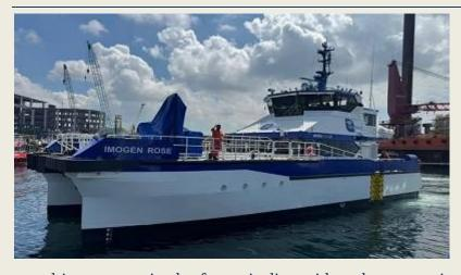
UK-based offshore wind crew transfer provider Tidal Transit recently added two catamaran crewboats in a series to its fleet of windfarm support vessels. Built in compliance with UK flag rules and Bureau Veritas class requirements, Anthea Luna and Imogen Rose boast hull designs and onboard systems ensure that they can retrofitted with electric
