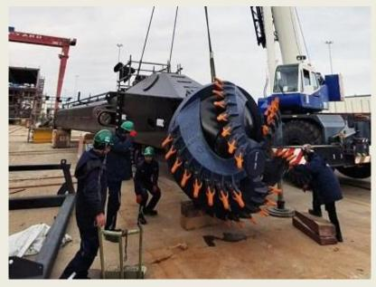
while the components for the second dredger were shipped from the Netherlands – assembled and commissioned at the Baku Shipyard LLC. The **CSD650** measures over 61 meter in overall length, has a hull length of 49.30m, a beam of 10.50m and draft of 1.65m. According to Damen, the newbuild will soon be performing various dredging jobs in harbors around the Caspian Sea. (Source: Dredging Today)
