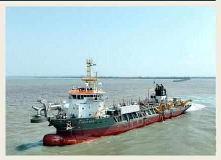
busy working in the ports of Chiapas and in Tampico, where severe siltation caused serious problems for shipping and commercial activities. The **Crestway and** its crew worked hard to complete these maintenance dredging works and ensure that both ports can continue their operations. Similarly the dredger will remove excess sediment from the Port of Tuxpan to create sufficient depth for ships calling at the port. (Source: Dredging Today)
