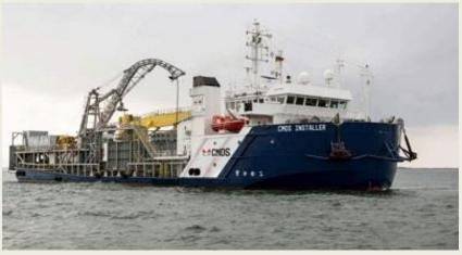
Bel Air, completing the offshore connection across Gorée Bay. Following the completion of works in Senegal, the vessel underwent a targeted upgrade program in Santander, which included carousel extension, ROV gate installation, and A-frame foundation improvements to expand its operational envelope for future scopes. **CMOS Installer** is currently engaged in export cable installation at one of Scotland's largest offshore wind projects, the 1.1 GW Inch Cape. (Source: Offshore Energie)
