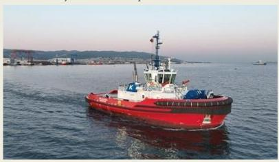
for five, for Kotug International's operations in West Africa. All are built to Robert Allan's RAstar 3200-W design with 80 tonnes of bollard pull coming from two Caterpillar main diesel fourstroke, high-speed engines turning two azimuth thrusters. They are set to support marine services at BP's Greater Tortue Ahmeyim (GTA) offshore project, which spans Mauritania
