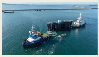
The commercial port's dry dock, now called "Forme Une," was inaugurated on February 21, 1913. dock suffered The extensive damage during the Second World War. After the end of the conflict, it was necessary to rebuild the gate boat. The latter, now nearly 80 years old, was showing signs of Brestport wear. therefore decided to replace it. The
