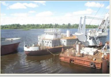
Kazakhstan. The vessel is being built to the RCO class - "P1.2". Paddle tugboat of the **TSK.566** project. Overall length - 44.8 m; Length on design waterline - 44.15 m Overall; width - 17.7 m Width on design waterline - 9.0 m; Height of the side at midship - 2.5 m; Deadweight - 44.55 t; Power - 800 hp. (Source: Sudostroenie; Photo: RCO)
