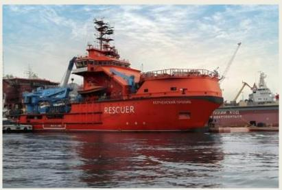
Specialists of the Amur Shipyard (part of USC) have started mooring trials the multifunctional rescue vessel of the MPSV 06 Kerch Strait project, which is being built by order of the Federal State Institution Directorate of the State Customer. During the trials, the main diesel generators (MDG) were started, operation of the integrated ship control system and its interaction with the MDG
