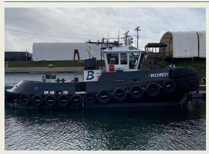
Longview, Washington-based towage company Brusco Tug and Barge has taken delivery of two new ship handling tugs in a series built by Diversified Marine of Portland, Oregon. Designed by Canadian naval architecture firm Robert Allan Ltd (RAL), Rascal and Rowdy each have an LOA of 65 feet (20 metres), a moulded beam of 32 feet (9.8 metres), a moulded depth of 11.5 feet (3.5 metres), and a gross tonnage of 159. The tugs were designed and constructed to comply with all
