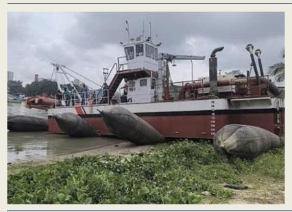
Dockyard and Engineering Works (DEW) has successfully launched its newly built Cutter Suction **Dredger 400**, developed with the engineering expertise and component support of Dredge Yard B.V., based in the Netherlands. The new dredger is equipped with a Mitsubishi engine, a hydraulic cutter head drive, and an inboard dredge pump directly mounted on a gearbox for efficient power transmission. Designed reliable and effective operation,
