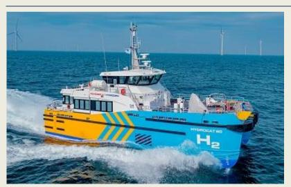
Dutch offshore support specialist Windcat Offshore has windfarm new crewboat into service. Hydrocat **60** is the second in a series of catamaran crewboats to be acquired by Windcat as well as the first of the series to be powered by hydrogen. With an optimised hull shape, increased beam, and elevated freeboard, the series was built to ensure accessibility greater
