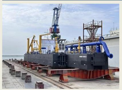
Damen is about to launch another cutter suction dredger from the CSD650 series in Azerbaijan. The latest CSD, built at the Damen Dredging yard in the Netherlands, has been transported to Baku Shipyard LLC for reassembly and delivery to a local client. Baku Shipyard is the perfect location for this task, as they have recently built another Damen CSD650 for local customer, the Engineer Soltan Kazimov. The CSD650 measures over 61 meter in overall length,
