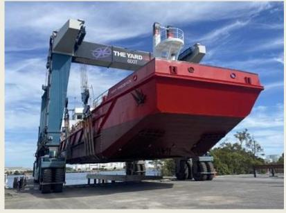
well prepared for her next dredging season. Built for precision and adaptability, the 50m Port Frederick is purpose-designed to operate where conventional dredgers can't—handling shallow-draft work, environmentally sensitive areas, and logistically complex sites. From regional port maintenance to remote marine infrastructure projects, this vessel leads McQuade Marine's fleet in both capability and reliability. (Source: Dredging Today)
