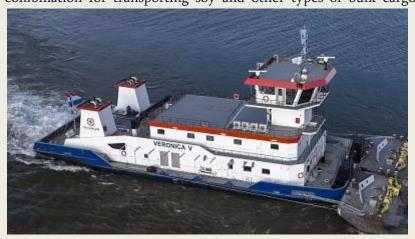
Rivers, where low water levels are a recurring challenge during the dry season. Thanks to their shallow-draught design, the vessels can maintain operations year-round, even when the water level drops to less than two metres. *Specifications* Type of vessel: Pusher tug; Classification: RINA; Lloyd's; Flag: Paraguay; Owner: Girona Rio Sur Transporte y Logistica,
