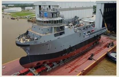
Shipbuilder Austal USA launched its first steel vessel, the future USNS Billy Frank Jr. (T-ATS 11), on June 14 at its shipyard in Mobile, Alabama. The ship is the first built using the company's new automated steel panel line. The 3,100-ton vessel is the heaviest ship launched by Austal USA to date. Billy Frank Jr. is the first of three Navy towing, salvage ships rescue (T-ATS) currently under construction at the shipyard. The vessel was over
