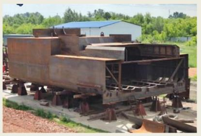
The Russian Classification Society (RCO) continues technical supervision of the construction of two T20 project pusher tugs. This was stated in a statement by the institution on June 13. The construction of the vessels is being carried out under the technical supervision of the Ob-Irtysh branch of RCO. The tugs are being built to class "P1.2 (ice 30)". Project T20 pusher tug. Overall length - 20.5 m Length; by design waterline - 20.29 m;
