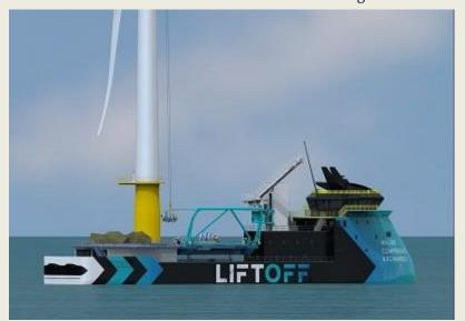
turbine maintenance, the **MCEV** combines LiftOff's proven up-tower crane technology with capabilities of modern offshore dynamically positioned (DP) vessels and mission equipment. LiftOff will offer turnkey services for major component exchanges using the MCEV. With a rapidly offshore expanding wind energy market, combined with an aging fleet of installed wind turbines, operators increasing delays due to limited
