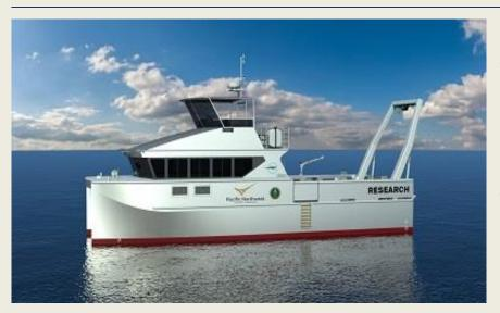
Seattle shipyard Snow & Company has started building a new 15m hybrid catamaran research vessel for operation by the Pacific Northwest National Laboratory. The Incat Crowther designed vessel will be powered by an advanced parallel hybridelectric propulsion system, consisting of two Volvo Penta D8-510 main engines, capable of producing 374
