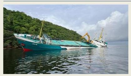
The Guyanese-flagged cargo vessel Hein (Imo 6702284) has partially submerged after running aground on the southern side of Monas Island. The incident occurred after the vessel's cargo of bricks reportedly shifted while en route to St. Vincent. To prevent capsizing, the crew made the decision to beach the vessel. Authorities have confirmed that there are no
