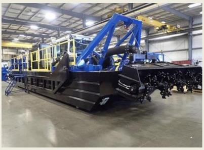
increases efficiency as there are no anchors or swing wires to manage. The 7012 HP is ideal for sand mining, reservoirs, marinas and ports, canals, mine tailings ponds, and large industrial lagoons. (Source: Dredging Today)
