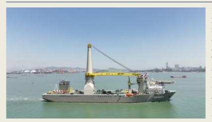
Bokalis's new crane vessel Bokalift 2 has set sail from Singapore to its first assignment on the Changfang and Xidao offshore wind farm project in Taiwan, where it will transport and install jacket foundations and the accompanying pin piles. The vessel was converted from a drillship (previously known as YAN) into a DP2 crane vessel at the Dubai-based Drydocks World,
