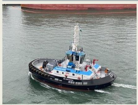
The Wilson Sons company began operating the first in a series of six new company tugboats. With Damen RSD 2513 design, the ship has a hull design that reduces greenhouse gas emissions by up to 14%, thanks to more efficient hydrodynamics. In detail, its twin fins would improve navigation increase its towing capacity during maneuvers, which would guarantee a reduction in fuel consumption and, consequently, in emissions. In addition, the new ships
