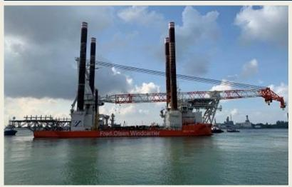
The new 1,600-tonne Huisman leg encircling crane on board Fred. Olsen Windcarrier's vessel **Bold** Tern has been commissioned, with the vessel now capable of installing wind turbines of up to 15 MW. Load testing of the crane was done earlier this month in Singapore, where the vessel was upgraded at Keppel FELS yard. Bold Tern arrived in Singapore in September 2021 to be fitted with the new
