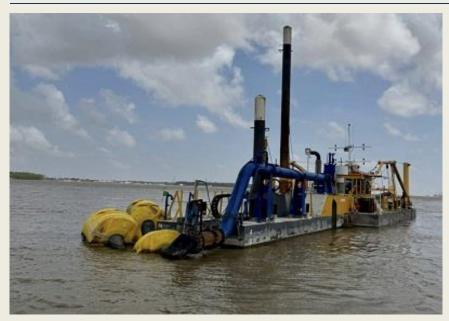
Guyana Port Inc. embarked on its first fullscale dredging campaign, powered by the CSD 350 Cutter Suction Dredger (Miss P Mud Shredder) and the split barge, Captain Virat. The stationary dredger was recently delivered by Damen with a comprehensive start-up package including floating pipelines, spare parts, and training. With a dredging depth of up to 9 meters and a production rate of 250
