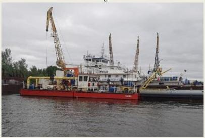
design waterline -7.268 m Height of the side at the midship -2.0 m Displacement of the vessel empty -113.59 t Deadweight -12.79 t Main engine power -650 kW Development depth -2-15 m Water productivity -2000 cubic meters/hour (Source: Sudostroenie; Photo: RKO)
