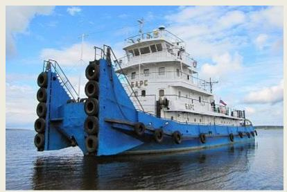
Let us recall that the tugboat **Bars** joined the Oboronlogistics fleet in early 2025 as part of the plan to enter the inland waterway transportation market. The **Bars** vessel is a twin-screw pusher tug and is designed to push sectional and barge trains, as well as tow barges. (Source: Sudostroenie; Photo: Oboronlogistics)
