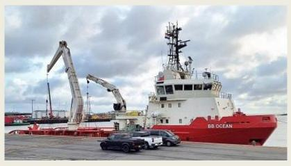
as a supplier, anchor handler and tug, among other things. The two cranes that are set up on the 372 square metre work deck can be used to carry out installation work. The ship was launched in 1999 at the Japanese Imamura shipyard in Kure and has since sailed under the names Pacific Supporter and Subsea Supporter. Since 2017, she has borne her current name and has Haugesund as her home port.
