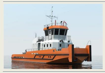
The R-Flot Group of Companies presented the technical design of the RPT2507 pusher tug. Details are given in the group's message dated June 10. As stated in the group's materials, the technical design developed was specialists from R-Flot. Design. The vessel meets the requirements of the Russian Classification Society (RCO) and the Russian Maritime Register of Shipping (RS). The pusher tug is designed for towing and pushing
