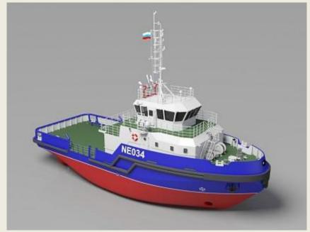
Nordic Engineering JSC have succeeded in a joint work on a concept design for а multifunctional tug of Arc 4 ice class, Project NE034. The design meets the requirements of Russian Maritime Register of Shipping and intended for insuring safe mooring of ships, providing assistance to ships of 201-220 meters in length, conducting and towing canting operations, firefighting, supply and oil spill response operations, hydraulic engineering and other works.
