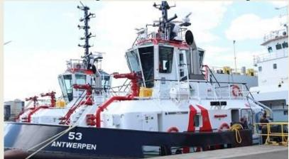
III compliance. RSD tugs are designed with а dual-bow principle, making them manoeuvrable and versatile for both forward and backward towing operations. In addition, Antwerp-Bruges Port of is converting further tugs to run on sustainable biofuels. The Tug Presentation Technical Tour was hosted by Port of Antwerp-Bruges, Damen, CMB.TECH and
