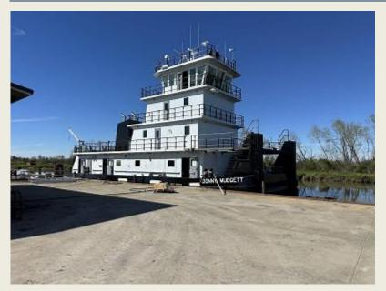
Hines Furlong Line has taken delivery of the M/V **Donny** Mudgett, the first vessel completed in its eleven-vessel newbuild program. Built at Intracoastal Iron Works in Bourg, Louisiana, the M/V Donny Mudgett is powered by three Mitsubishi Tier S6R2-3 Y3MPTAW engines, each delivering 803 horsepower at 1,400 RPM. Donny Mudgett is the first of eleven vessels currently under construction at Intracoastal Iron Works and Eymard Marine Construction &
