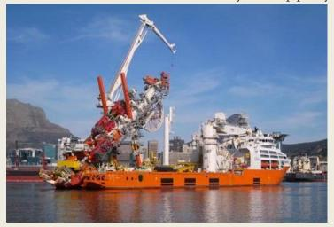
operations, with the tower able to be angled anywhere between 40° and 90°, allows **'Shen Da Hao'** to lay pipes up to a depth of 3,000 metres. She is able to operate almost anywhere on earth, as she has an ice classification of ICE C, which allows her to operate in Baltic Sea first year ice thickness of up to 0.4 metres. When utilised as a heavylift crane vessel, she is fitted with an NOV active heave compensated (AHC)
