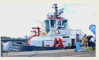
built RSD 2513 tug with batteries and genset back-up. It was delivered to Port of Antwerp-Bruges in
