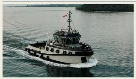
Indonesian shipbuilder KTU Shipyard has completed its first harbour tug built in collaboration with naval architects Robert Allan Ltd at its Sagulung yard. It delivered 27-m Karya Pacific **2232**, an azimuth stern drive (ASD) tug built to RAL's TRA2700 design, to its own subsidiary Karya Pacific. Launched mid-April, this is the first of a new series of
