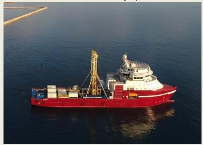
the subsea terrain for wind turbine foundations. Geoquip underwent thorough soil sampling seismic and site monitoring to inform the engineering parameters for both projects in depths of 40 metres. By deploying the Dina Polaris vessel, equipped with geotechnical drilling, sampling and testing equipment along with an offshore laboratory, Geoquip accurate, real-time provided identifying seabed data, challenging site conditions safely
