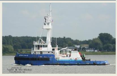
twin screw tug was built in 2003 by Stoc.Kozle Serwis in Poland and Damen Hardinxveld in the Netherlands. Meanwhile the company is shedding three of its older tugs which have not been operational for several years. These include: 1. **Océan Echo II** This twin screw 3,000 bhp veteran tug was built in 1969 by Port Weller Drydock for Atlantic and Pacific Barge Transport Ltd. Named Atlantic it was contracted, along with two 7850 ton deadweight barges built in the same yard, for a
