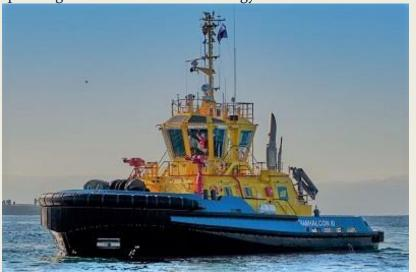
where Saam operates. Saam Halcon III has an LOA of 24.4 metres, a moulded beam of 11.25 metres, and a maximum operating depth of 5.6 metres. Power is provided by two Caterpillar 3516C engines connected to Kongsberg US205 fixed-pitch azimuthing thrusters. The engines each produce 2,100 kW at 1,600 rpm to deliver a bollard pull of 70 tonnes and a free
