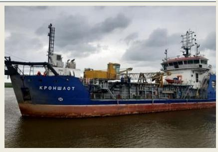
m; Hopper capacity - 1000 m3. Class notation: KM Ice1 R1 AUT2 Hopper Dredger. The TSHD 1000 series vessels are able to dredge to a depth of 20 meters and operate at water temperatures -2 ° C to + 20 ° C. (Source: Dredging Today)
