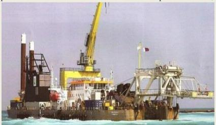
the unused capacity of the electrical installations to the maximum within all safety margins. Upgrading the pump power from 6000 to 7400 kilowatts allows the vessel to move large amounts of sand over large pressing distances quickly," said project manager Arie de Jong. Under the contract, Bakker Sliedrecht also updated all automation systems, inspected electrical
