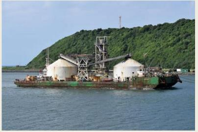
minerals, with the loading gantries used for the actual transhipment. The vessel is selfpropelled for the jetty-bulker shuttle (although she did not use her own propulsion capability for the Moma-Durban voyage), with a designated carrying capacity of just over 5,000 tons. That equates to a very large number of shoreto-ship cycles, as the Kenmare mining website reflects annual exports of something in excess of 800,000 tons. It is not clear
