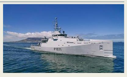
country's capability to respond effectively, rapidly and cost-effectively to threats such as illegal trafficking and fishing. The 62m by 11m vessels have been designed by Damen to deliver a rapid
