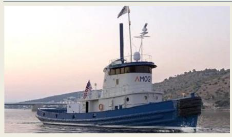
C-Job Naval Architects will integrate Amogy's ammonia-to-power system into the existing tugboat and lay out the framework shipyard activities, including retrofitting construction, engine removal and outfitting associated equipment and After machinery. conversion project, this tug provide
