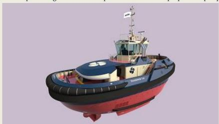
the thrusters are mounted side by side, and overall brings a significant increase in stability and freedom of movement. As a result of these features. the TRAnsverse tug meets the full range of complex harbour terminal and towage environments, providing benefits such as the ability to reduce overall time of tug jobs, greater
