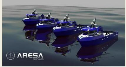
The ARESA 2500 S RWS is a semi industrial seiner fishing vessel which integrated a suction modern fishing system and RWS Refrigerated Water Systems in the fishing holds. With 25 meters of total length have a capacity of 50 tonnes of fish in the holds. The ARESA 2500 S RWS is the evolution of the successful model ARESA 2500
