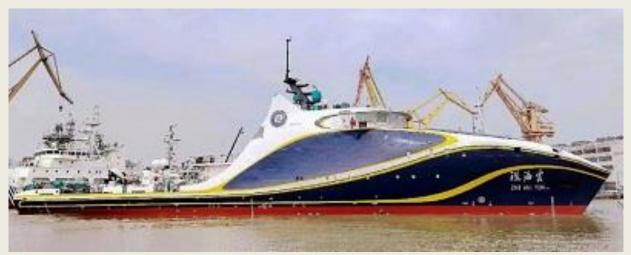
one 1,140kW generator, two 1,950kW azimuth pod thrusters, and emergency use batteries with a total output of 600 kWh. The vessel will be operated as a large mothership for unmanned research craft. *(Source: Baird)*
