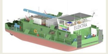
freight lighter, URSUS. Therefore, along the shipping routes of Berlin towards Rhine/Ruhr, Hamburg and Stettin, there will only be one additional shore station required to provide **ELEKTRA** with hydrogen and electricity aside from Westhafen. In all, convoys of up to 150m long can be driven. Both in
