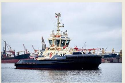
Sanmar Shipyards has delivered a powerful and highly manoeuvrable new build RAmparts 2400SX class Z-drive tug to global towage giant Svitzer, which will join its operations in the Dominican Republic. SVITZER RIVAS, known as Bogacay XLVI while under construction at Sanmar's purpose-built shipyards in Turkey, is the 27th tugboat that Sanmar has delivered to world's largest the tug
