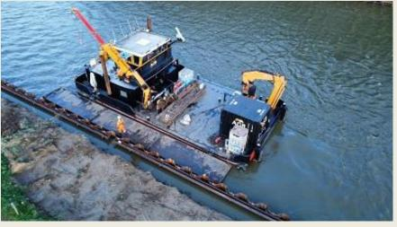
its push bow. The vessel has a 60-ton-metre crane for heavy duty work and a 26-tonne crane for auxiliary jobs. At 18.80 x 8.20 m, it is a compact boat (with a very low draught), but it has everything on board to get the job done. Apart from the cranes, for example, it also has a moonpool, two 80-
