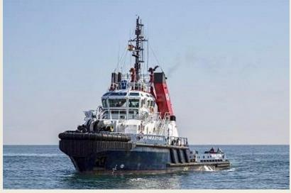
Shipyards and in service since 1998. It is also a powerful vessel in its category, powered by two Mak 8M20 engines with a power of 4,200 horsepower, in a hull 28.50 m long and 11 m wide. The draft power of it is 51 tons. (Source: Puente de Mando; Photo: Antonio Alcaraz Arbelo)
