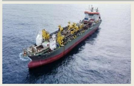
Keppel Shipyard has completed the lengthening of Boskalis' trailing suction hopper dredger (TSHD) Oranje from 156 to 201 metres. The length extension project follows the similar extension of Boskalis' hopper dredging vessel Prins der Nederlanden, which conducted in the first half of 2022. The conversion involved mid-section restructuring by insertion of
