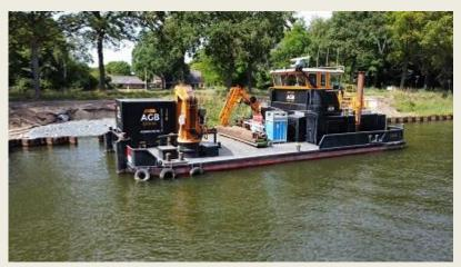
Contracted by the Van Oord-Hakkers-Beens combination, workboat Destiny proved itself as a true multifunctional platform. After 17 months of canal quayside towing and pushing, work, welding and cutting and various additional jobs, the job is done for the crew and their special vessel multipurpose work 'Destiny' of AGB Maritiem. The pusher/'multicat' vessel was part
