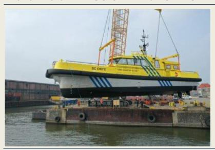
Last week we launched the SC ONYX for Sima Charters with our Liebherr 1300 at our Merwede Yard. With a lifting capacity of almost 300 tons this vessel was an easy job for our crawling crane. The vessel will be prepared for her sea trials end of this week. We would like to thank Sima for the good cooperation. (Source: Neptune)
