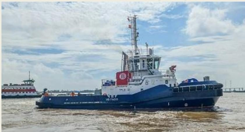
Svitzer has taken delivery of the first of two tugs ordered from Turkish builder Med Marine in February of this year. The Robert Allan Ltd-designed, 28- by 13-metre tug has a bollard pull of 75 tonnes and a speed of approximately 12 knots. Duties will include escort and firefighting in Suez Canal waters. The second tug
