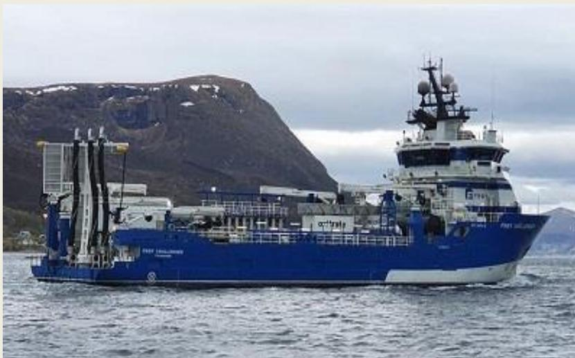
A vessel that was originally built for offshore platform supply duties has completed undergoing conversion work in preparation for its new role as a fish delousing boat. Owned by Norwegian aquaculture support company Froy Gruppen and operated by its subsidiary Froy Akvaerssurs, ex-**Skandi Texel** was formerly owned by offshore specialist DOF in support of customers in the oil and gas sector following its
