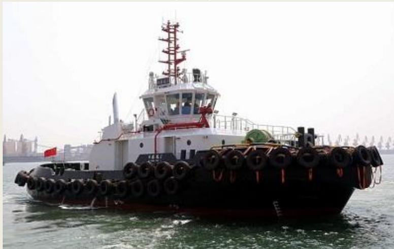
local branch of Boluda France. **VB Likurai** and **VB Fado** each have a length of 30.3 metres a moulded beam of 10.4 metres, a maximum draught of five metres, and a bollard pull in excess of 45 tonnes. Accommodations are available for six crewmembers. The tugs will be capable of “push/pull” towage and will be used for both harbour and deep-sea operations. *Svitzer's newest tug to be deployed for Suez Canal towage duties*
