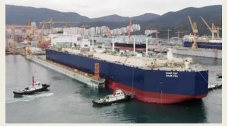
Yamal, а fleet of 15 icebreaking LNG tankers were constructed between 2016 and 2019, to be able to export LNG year round from both Yamal, which became operational in 2017, and the new Gydan LNG field. These specialised icebreaking LNG tankers, which are of ARC7 classification, and capable of breaking ice that is 2 metres thick, will export the LNG
