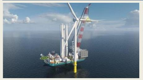
NOV has once again signed contracts with CIMC supply Raffles to а GustoMSC<sup>™</sup> NG-20000X self-propelled wind turbine installation jack-up vessel Havfram's design for second vessel on order at the shipyard. The NG-20000X-HF vessels are among the largest wind installation jack-ups in the industry, NOV said. They
