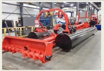
Mud Cat has just shipped another Mud Cat MC 100E dredge to a contractor in Texas. The MC 100E hull is of heavy-duty constructed gauge steel, never poly plastic floats, and will not crack when exposed to variable pН environments combined with heavy UV exposure. According to Mud Cat, the 100E is the most powerful radio remote controlled auger dredge on the market today. Also, this remoted controlled dredging
