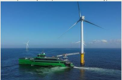
**Aqua Helix** for crewing transport solutions from the Dutch shore to offshore installations in the North Sea. Weight reduction is key if a ship needs to sail at high speed. The slender hull of the FCS 7011 is built in aluminium. quest for lightweight construction has led increasing the hull sides upwards along the accommodation decks, add to structural they integrity. This way, less heavy structural beams are necessary.
