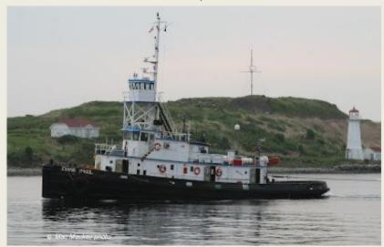
equipped with an Ingersoll Rand D-E plant with two 6 cylinder, 500 bhp Ingersoll Rand diesels, each with 50 kW generator A single screw tug, it was 111 ft long x 25.6 ft breadth, and was intended for barge work with a heavily fendered hull. (Many railroad tugs in New York harbour were also diesel-electric and the Canadian Pacific Railroad had its own D-E tug the **Prescotont** in barge service between
