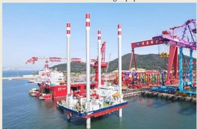
movable drilling position in a arrangement triangular digital assistance for the drilling controls to improve accuracy and efficiency. The arrangement of the drilling positions also enables the platform to conduct soil layer analysis and exploratory drilling at the same time. The drilling equipment will also be used for sampling, dynamic penetration, standard penetration. A and moonpool is also installed. The main platform assembly is elevated
