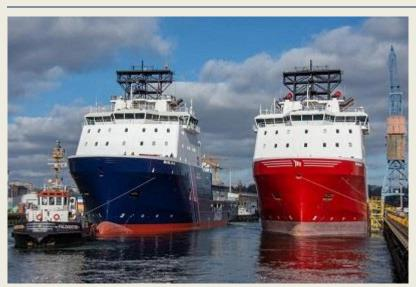
German Naval Yards has converted and and will delivery later May the highin tug **Abeille** performance Normandie to the French shipping company Les Abeilles. The vessel arrived at shipyard for conversion in September 2021. The 91 x 22-m vessel has a 282 ton towing capacity and 20,800 kW (28,300 hp) of power, and will be available to the French Navy as a multifunctional emergency tug.
