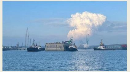
The first of 23 caissons for the foundation of the energy island in the Princess Elisabeth zone has been placed. The concrete colossus was towed this week from the construction site in Vlissingen to its destination 45 km off the Belgian coast. The Common Nautical Authority which manages shipping traffic Scheldt the Western on between Belgium and the
