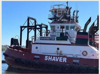
replacement of the tug's main engines and installation of new drives, delivering increased bollard pull and improved responsiveness. Caterpillar 3512E main engines rated at 2,549 BHP will be coupled to Berg MTA 524 drives. To further optimize the vessel's capabilities, Glosten performed a complete redesign of the pilothouse to improve visibility from the main operating station. The new pilothouse will feature larger windows and expanded sightlines—particularly toward the working
