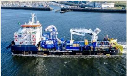
campaign will happen during the summer and will be carried out by the company's cable repair vessel Curo. The vessel is equipped with an eight-point mooring system that allows it to maintain position during operations, even in strong tidal conditions. It also has beaching capabilities, which enable the vessel to safely approach and work as close as possible to the landfall location. *(Source: Splash24/7)*
