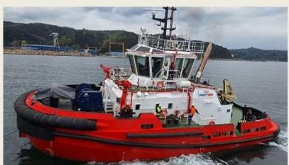
ship fire-fighting system. Med Marine launched newbuild ER172 on 12 February 2025. It was built to a Robert Allan Ltd RAmparts 2500-W design with twin diesel engines driving Z-drive azimuth thrusters through dedicated shaft lines. Med Marine said this tug will handle a broad spectrum of
