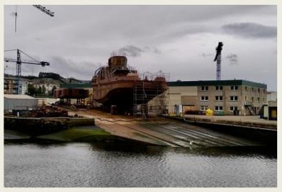
The launch of Armón Navia Shipyards' 869th construction, the ASD Schottel tugboat "Treintaysiete," is scheduled for next June. The tug is currently in the slipway and will be delivered next September. Built to order by Remolques Unidos (RUSA) of Santander, this is a 490-gross-ton azimuth tugboat with a hull measuring 32 m in length and 11.70 m in width. It will be propelled by two engines with a combined output of 6,868
