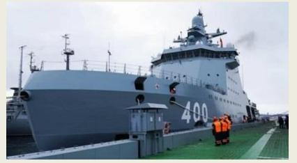
begun testing its first "combat icebreaker," a rare gray hull vessel purpose-built for Arctic service. The newly-delivered **Ivan Papanin** is the first of two Project 23550 conventional icebreakers delivered by United Shipbuilding Corporation (USC) for the Russian Navy's Northern Fleet. It launched in 2019, began sea trials last year and has now completed ice testing in
