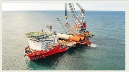
After all 95 installing monopiles at Dogger Bank B, the offshore installation vessel Seaway Strashnov has moved on to the third phase of the UK's Dogger Bank Wind Farm, where it has now begun foundation work at Dogger Bank C. Seaway Strashnov and Seaway Alfa Lift commenced the installation work at Dogger
