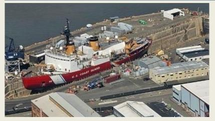
The Coast Guard has initiated the final of five planned phases of the service life extension program (SLEP) for Coast Guard Cutter Polar Star, the service's operational sole heavy icebreaker. Polar Star arrived at Mare Island Dry Dock in Vallejo, California, on March 30 to begin the remaining SLEP activities. The work is part of the In-Service Vessel Sustainment
