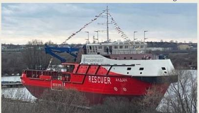
superstructure. The accommodation is located in the bow of the vessel, the engine room is in the middle. The vessel is equipped with two propellers, two bow and one stern thrusters. Multifunctional emergency rescue vessel of the MPSV12 project. Class symbol − KM → Arc5 (hull; machinery)[1] AUT1 FF2WS DYNPOS-2 BWM(T) DETier III Salvage ship Oil recovery
