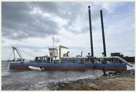
Oiltech Dredging Equipment, in collaboration with Impianti Draganti, has successfully delivered an overhauled IHC Cutter Suction Dredger (550) to a client in Africa. Together with Impianti Draganti, the company carried out a comprehensive overhauling of the dredger. The new Caterpillar 3512 engine was installed to replace the one, existing ensuring optimal performance and
