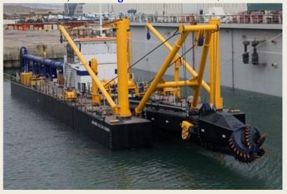
CSD measures 61.20 meters in overall length, with a hull length of 49.30 meters, a beam of 10.50 meters, a draft of 1.65 meters, and a maximum dredging depth of 18 meters. Remaining commissioning and sea trials are scheduled to be carried out at the outfitting quay of the Shipyard. (Source: Dredging Today)
