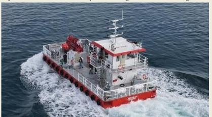
infrastructure, buoy maintenance, the lifting of moorings, the transport of equipment, and towing operations. Compliant with IMO Tier III standards, the 12tonne bollard pull Langilea is equipped with catalytic reduction systems with urea injection reduce to **NOx** emissions. The vessel is fitted with two cranes, a 30 tonne-
