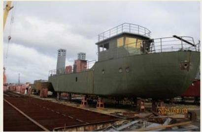
A". Self-propelled oil recovery vessel of the TSK.580 project: Overall length m 25.5 m; Length on design waterline - 24.8 m; Overall width - 6.3 m; Width on design; waterline - 6.0 m Height of the side at midship - 2.7 m; Freeboard height - 1.08 m; Deadweight - 6.49 t; Displacement - 174.49 t. *(Source: Sudostroenie; Photo: RCO)*
