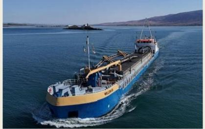
has a shallow draft and good maneuvering properties thanks to the twin-screw propulsion and a powerful bow thruster. This allows the TSHD to carry out dredging work in shallow water and/or tight places. Also, the Willem Sr is equipped with a drainage system. According to Filia, this system extracts the water from the cargo, after which it can be unloaded dry by a shore crane. *(Source: Dredging Today)*
