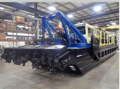
dredger is capable of cutting vegetation with the optional patented WeedMaster® cutterhead, IMS said. *(Source: Dredging Today)*
