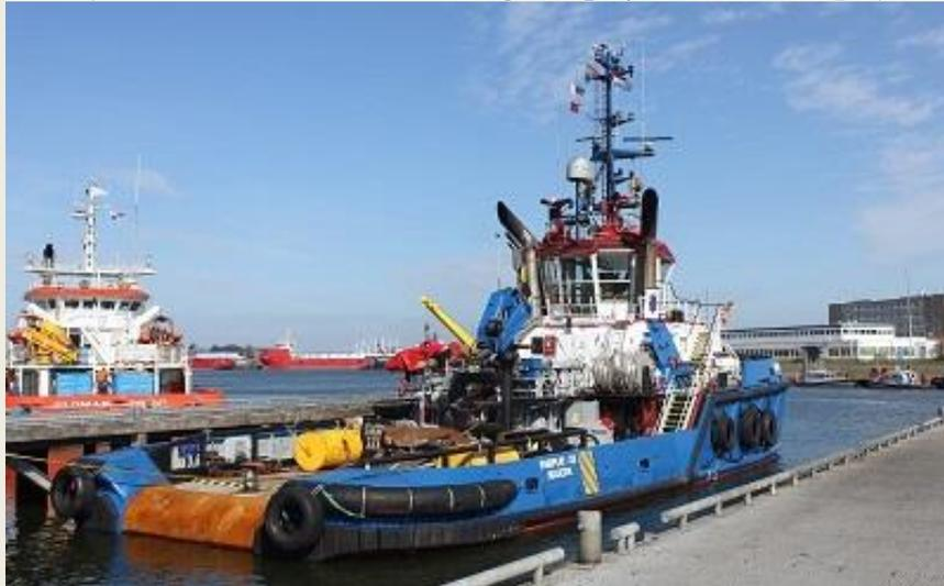
sturdy tug, with a pulling power of 75 tons, which had recently moved Valaris 120 in the British sector of the North Sea oil rig. In addition to towing and recovery, the **Fairplay-33**, built in 2006, can also be used for escort services and as a firefighting vessel. The tug still sails under the Portuguese flag and has Madeira as its home port.
