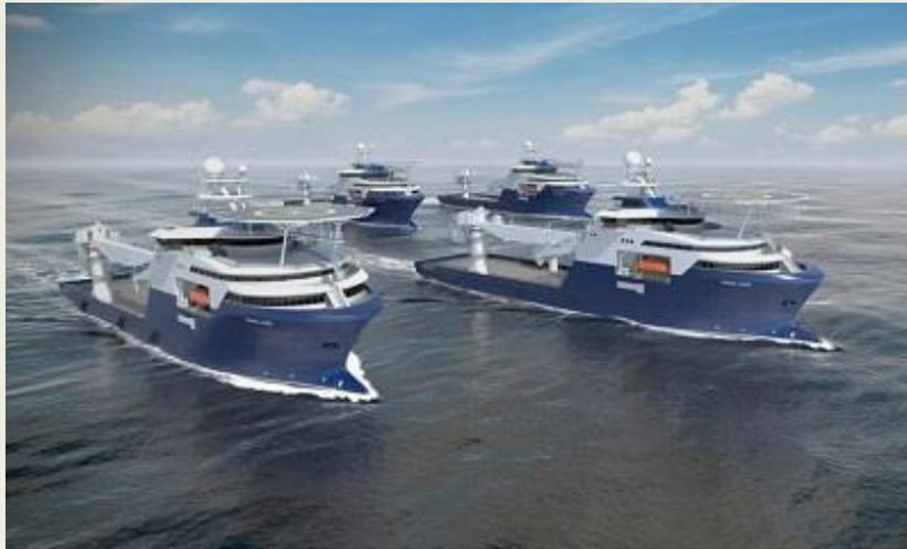
for an undisclosed price tag, will be mainly used in traditional oil and gas and offshore renewables sectors. The 100-m-long units have been designed by Norway's Salt Ship Design as a further development of the Salt 305 vessels previously built by the same yard. The new design, dubbed Salt 0494, is prepared for alternative fuel and includes a large battery
