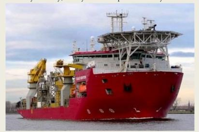
build bespoke sophisticated vessels that specialise only in those construction and maintenance elements that are present in the oil and gas industry, so it would not surprise anyone to learn that the wind power industry also build vessels that are unique to their needs. On 14th March, at 15:00 in the afternoon, the cable laying vessel 'Isaac Newton' (IMO 9707297) arrived off Cape Town, from Zeebrugge in Belgium, and entered Cape Town harbour. She
