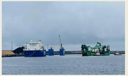
The Alvargonzález Group has managed the boarding operation in the port of El Musel of the French flag dredger "D' Artagnan" (IMO 9312963), which has arrived from La Pallice, for its transfer to Singapore aboard the cargo ship special "GPO Saphire" (IMO 9760445). The maneuver was carried out on the docks of the expansion of the port of El Musel, where there is sufficient
