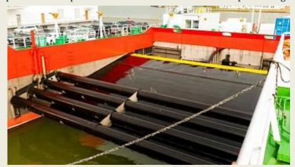
floats of the catamaran and is transferred into the wing tanks in the floats, where oil is separated by gravity from the water. The water is then transferred into the lower part of the tanks, while the oil is kept in the tank because of its lower density. **Westensee** can skim around 90,000 m<sup>2</sup>/hr at a speed of 3 knots. It is stationed in Bremerhaven and can be mobilised into the North Sea or
