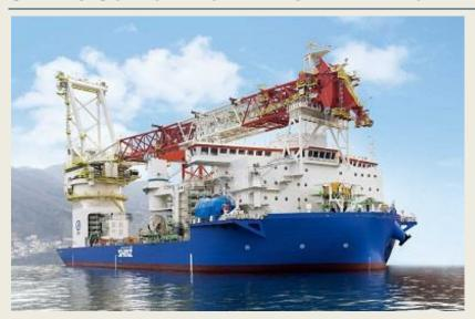
The Japan Marine United (JMU) shipyard delivered the **GustoMSC** designed and equipped offshore wind turbine installation vessel (WTIV) to Shimizu Corporation at the end of January. Shimizu unveiled plans to build a wind farm installation vessel back in 2019. The vessel, which GustoMSC SC-14000XL design, is 142 metres long, 50 metres, wide, and can accommodate up to 130 personnel. It is also
