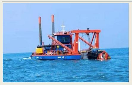
Two units of heavy-duty large capacity HID Brand CSD will be used for hard materials dredging such as harsh sand and gravel in Abu Dhabi for the purpose of the Army Port construction project. The cutter head power is 700KW, flow capacity is 700m3/H with a dredging depth of 18m. The dredger is equipped with DGPS system to monitor and prospect the underwater dredging areas. "This piece of
