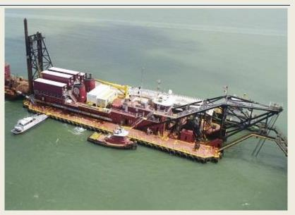
Corporation used their cutter suction dredge Alaska to accomplish the work. The dredging, which kicked off in early February, removed approximately 200,000 cubic yards of sand from the port's channel and turning basin. The sand was placed on the shores of the Town of Palm Beach, at no cost to the residents. (Source: Dredging Today)
