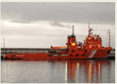
and as it is. Built in Huelva Shipyards and in service since 1982, it is a ship of 1,171 gross tons in a hull 62 m long, 11 m wide and 5 m draft. Two diesel engines allow it to maintain a speed of 16 knots. (Source: Puente de Mando; Photo: Celso Hernández)
