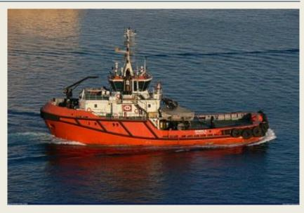
powered by two MAK 8M25 engines that total 7,180 horsepower and drive Voith Schneider propellers. It is also equipped with three auxiliary motors of 150 kW each. Of 701 gross tons and 300 tons of dead weight, it measures 36.65 m in length, 13.60 m in width and 6.60 m in draft. IMO code 9495258. (Source: Puente de Mando; Photo: Sydney Sinclair)
