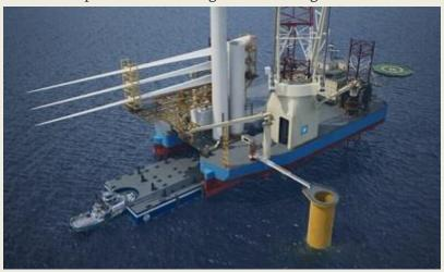
will render the work far less dependent weather on conditions, thereby reducing the number of operating required to install a wind farm. "Maersk Supply Service's new installation concept can make offshore wind farm installations significantly faster with estimated efficiency gains of 30%. The partnership with ECO makes this new technology available for the US offshore wind
