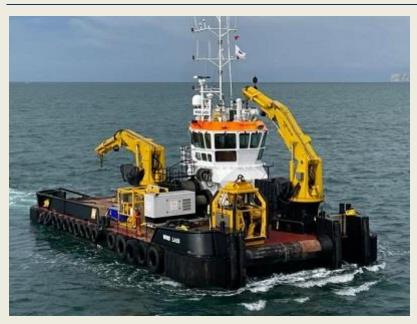
Landfall is expanding it's fleet with a fantastic shallow draft multipurpose workboat with a Bollard Pull of 37,2 T. The two strong HEILA marine deck cranes with a maximum lift capacity of 10,0 tons(m) at 16,5 meters, the waterfall double drum towing/anchor handling winches of 50 and 100 tons. Wind Lass The "WIND LASS", built in 2011, is a shallow draft multipurpose workboat of 26,00 by 11,50 meters. The twin Caterpillar engines delivering 1.902 kW which results in 37,2 tons bollard
