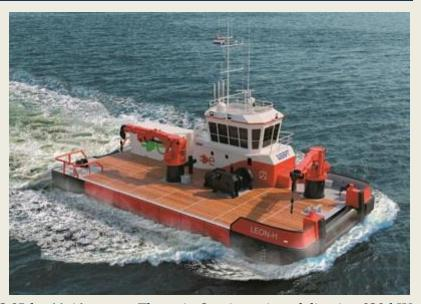
draft multipurpose workboat of 23,95 by 11,46 meters. The twin Scania engines delivering 930 kW
