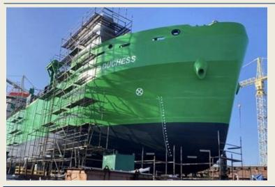
Neptune Marine continues to make great progress on the construction of PD Ports' new hopper dredger, the **Emerald Duchess**. The 71m long dredger will soon be launched (Q2) and put through the paces in the Netherlands. The 2.000m3 TSHD has been designed and built to an exacting specification to ensure it can carry out its tasks on the Tees to the highest environmental and safety standards. Also, the new vessel has been 'future-proofed' with a number of bespoke
