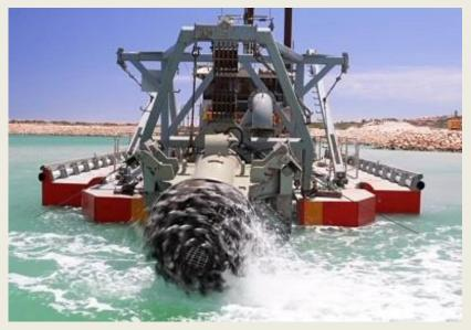
The dredging operations at Ocean Reef Marina, collaboration with the WA Department of Transport, are making great progress. According to the Ocean Reef Marina, the crews are on track to wrap up this phase of work in just a few weeks. Working on the project, the 22m cutter suction dredge "Cooper II" has encountered more hard rock deep in the marina basin, and this has meant the dredging is taking longer than anticipated.
