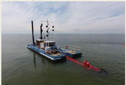
navigational projects locations such as small ports, rivers, and inland waterway dredging project. According to Ellicott, the dredge will be used for keeping navigation channels open and for supplying sand to help with erosion on the beaches along the York County coast. Several harbors and rivers along the York County coast will require maintenance dredging to ensure that the channels are navigable for
