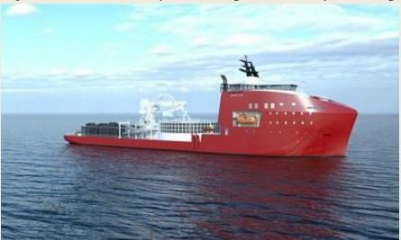
will be built entirely by Vard network, the including main the systems and equipment. It will have a length of around 95 m and a total of 3,700 tonnes of cable installation equipment. The shipbuilder said the vessel will deliver in 2024 and be able to reach a speed of 14 knots, and stand out for the solutions installed board.
