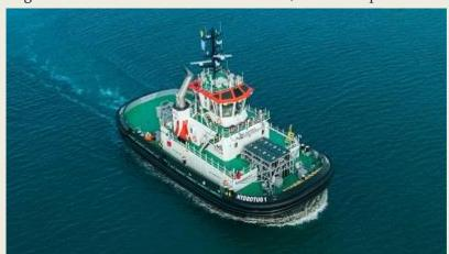
2024 for an unnamed client and has an order for another 32-m scheduled for delivery tug, December 2024 undisclosed owner. Armon Navia completed a world-first hydrogen-powered harbour tug in 2022 when it delivered Hydrotug 1 to the Port of Antwerp-Bruges. This 4,100-kW, 496-gt tug was developed by CMB.Tech with two BeHydro V12 dual-fuel, medium-
