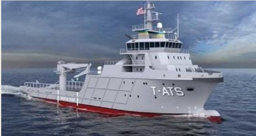
salvage, and rescue ships will be designed to support the navy's fleet operations. Each T-ATS will have a multi-mission common hull platform capable of towing heavy ships. The vessels will be capable of supporting a variety of missions including oil spill response, humanitarian assistance, search and rescue (SAR), and
