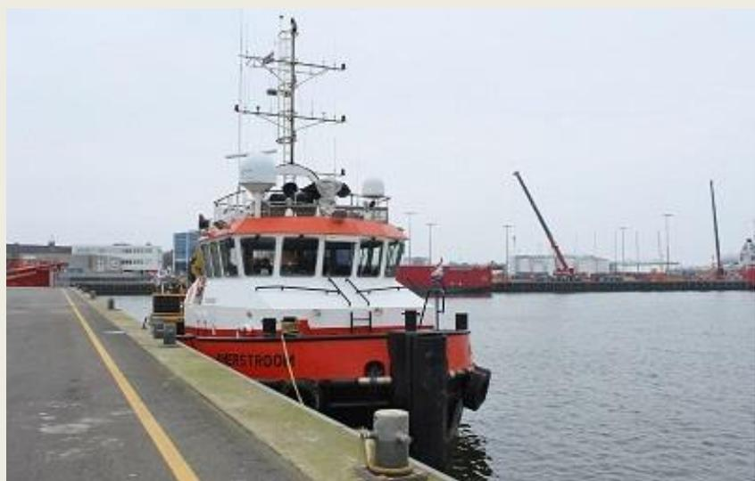
propulsion consists of two Caterpillar diesels of 485 hp each, which together provide a pulling power of 16 tons. The fleet of the shipping company from Hardinxveld-Giessendam currently consists of nine tugboats, three multcats, two pontoons and related equipment. Last month it was exactly fifty
