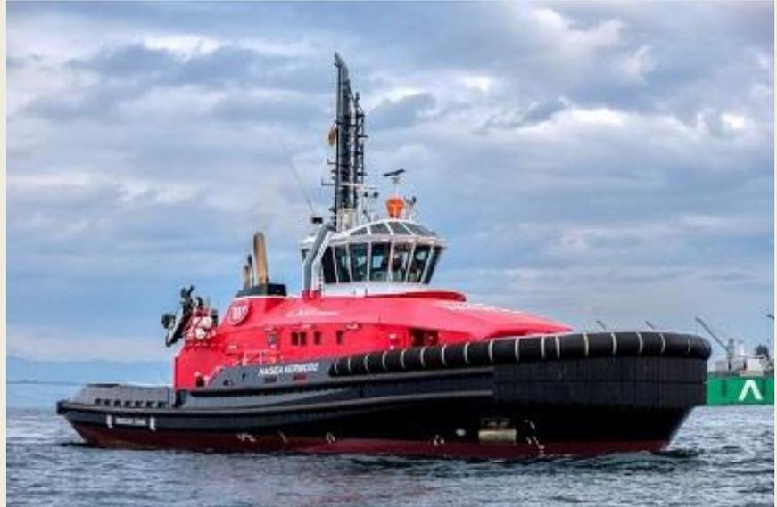
HaiSea Marine, Canada; Designer: Robert Allan Ltd, Canada; Length overall: 40.2 metres; Beam: 16 metres; Draught: 7.1 metres; Depth: 6.0 metres; Gross tonnage: 996; Bollard pull: 100 tonnes; Interior fitout: Toilets; Types of fuel: LNG; diesel; Accommodation: Cabins; Operational area: British Columbia, Canada. (Source: Baird)
