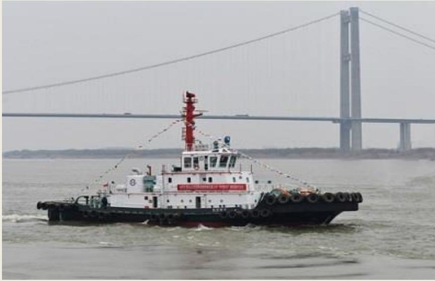
On 6th March, 2024, one unit 3,824 kW ASD tugboat built by our company Jiangsu Zhenjiang Shipyard for domestic shipowner has been delivered and sailed smoothly. The tugboat's overall length is 37m, the width is 10.6m, the depth is 4.9m, ahead bollard pull is 61.8t and astern bollard pull is 57.5t, and the speed is 13.85Kn. (Source: Jiangsu Zhenjiang Shipyard)
