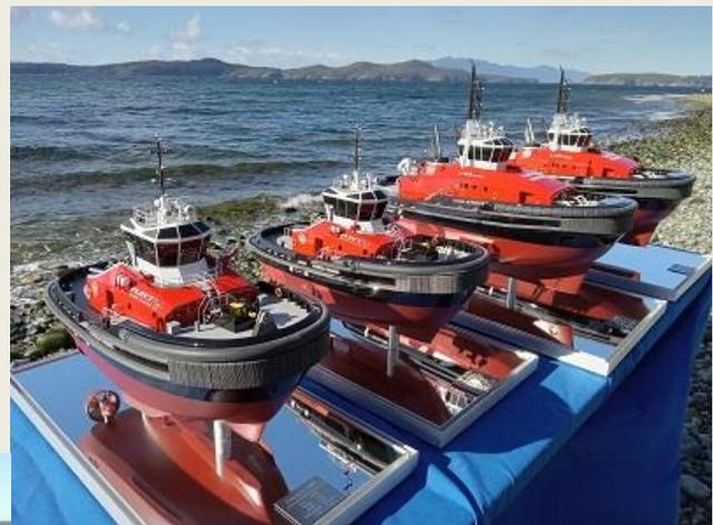
Haisea Kermode models depict the 40m RStar 4000 DF dual fuel escort tugs running on LNG or diesel. The three Haisea Wamis models depict the 28m ElectRA 2800 battery electric harbour tugs. The models feature fiberglass hulls, real rubber fendering all around, non-skid decks, soldered railings and many hand made, cast, and laser cut components...all created in house. The Models are made by Brian Klassen <http://www.brianklassenmodels.ca/>
