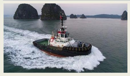
NEC has opted for IMO Tier III compliance in line with its values. National Energy Corporation (NEC), а subsidiary of the stateowned National Gas Company of Trinidad and Tobago, has taken delivery of a new Damen ASD Tug 2811. NEC has opted to have installed a Class certified Damen Marine NO x Reduction System to make it
