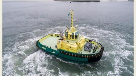
2,525 kW at 1,800 rpm, driving two Kongsberg Maritime azimuth thrusters of type US 255 P30/P35 with fixed-pitch propeller а diameter of 3,000 mm. During sea trials, Mai Koko achieved bollard pull ahead of 81 tonnes and bollard pull astern of 75 tonnes, speed ahead of 13 knots and astern of 12 knots. With the same propulsion equipment, Da-
