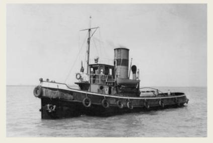
In February 1929, Compañía Remolcadores Valenciana de contracted the construction of the "Angela Comes" tugboat with the Unión Naval de Levante shipyard, which was the first in the history of the aforementioned factory. The keel was laid on January 31, 1930, the following August 10 it was launched and on September 25 of that year it was delivered to its owner, after carrying out the official sea trials, in which it reached a speed of 10.15 knots. It
