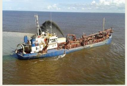
undertaken twice a year at the Port of Bunbury. A trailer suction dredge removes naturally accumulated sand and silt from the shipping channel and outer harbour berths, and deposits the material at the ocean spoil ground. *(Source: Dredging Today)*
