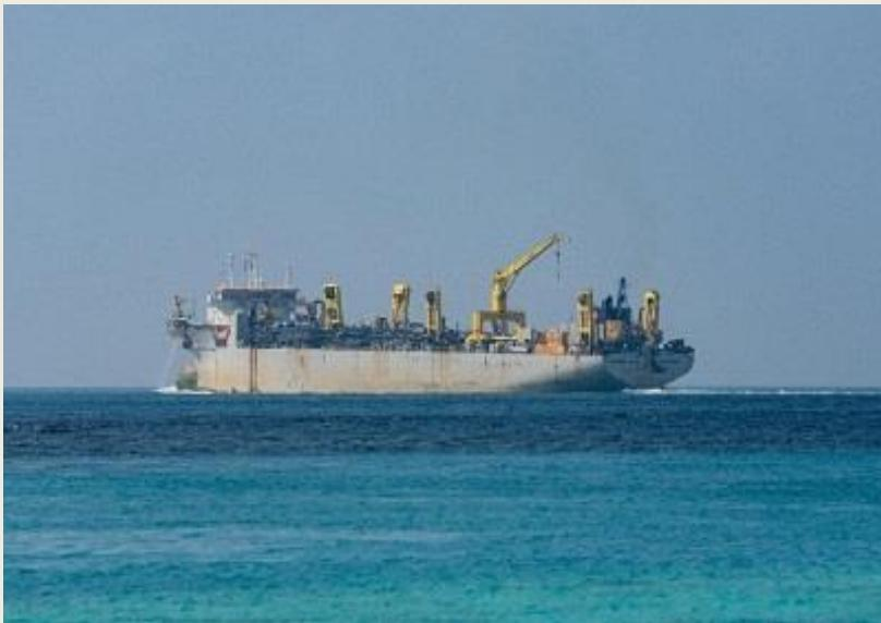
Maldives Airports Company Limited (MACL) said that a total of 116 out of 137.5 hectares have been reclaimed at Rasmalé Site A, reaching 84% completion. Reclamation works at Rasmalé Site A on started on December 1, 2025. The operations are being carried out with the Jan De Nul's trailer suction hopper dredger (TSHD) **Cristóbal Colón**. Rasmalé, also known as Maldives Eco City, is a groundbreaking project located
