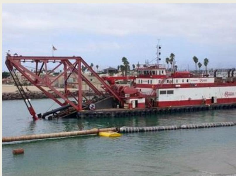
results from the down coast movement of an average of about 500,000 cubic yards of sandy material each year which is deposited by littoral processes in the sand trap and entrance channel. If this material is not dredged and deposited on the down-coast beaches, the harbor entrance can become unsafe for vessel navigation and the beaches are not adequately renourished. (*Source: Dredging Today*)
