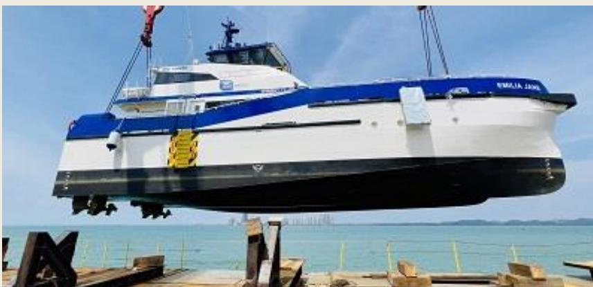
the latest WindFlex-27 with quad-IPS propulsion, designed by Incat Crowther UK and built by Penguin International Limited. Expected to arrive in the UK in March 2026, **Emilia Jane** will provide essential service and maintenance support to offshore wind operations in the North
