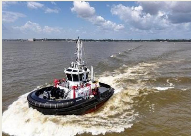
the last tugboat of a series of three new vessels built at the Rio Maguari Shipyard (ERM) in Pará. The company's most recent tugboat, the **SN Acaraú**, was delivered by ERM last year, with a Robert Allan design, Rampart 2300, with more than 75 tons of bollard pull (BP), Kongsberg azimuth thrusters and two Caterpillar engines. This +75 BP tugboat also has a FiFi 1 (firefighting) system. The next unit to be delivered will reinforce the company's
