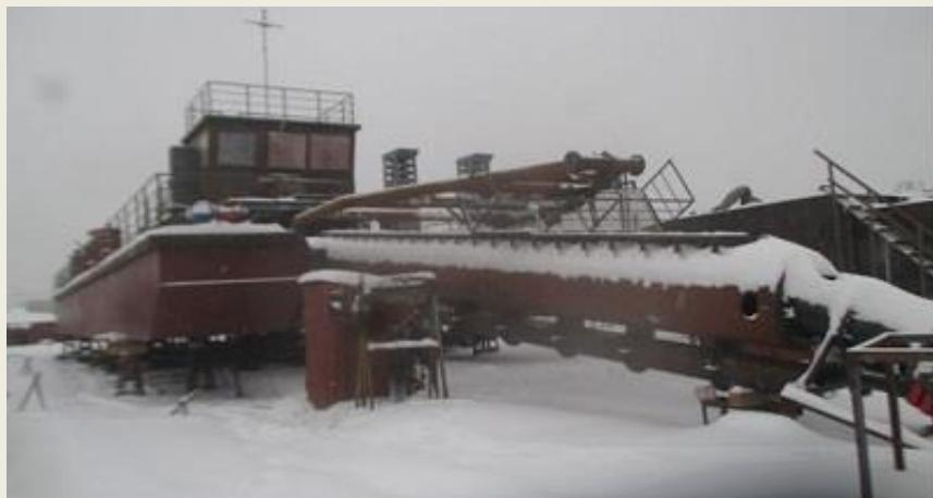
project TSK.571; Overall length – 32.0 m; Length on design waterline – 31.63 m; Width on design waterline – 10.04 m; Height at midships – 2.0/3.4 m; Deadweight – 35.36 t; Gross tonnage – 76.10 m; Development depth – from 1 to 13 m; Productivity on soil – 833 m<sup>3</sup>/h. (Source: Sudostroenie; Photo: RKO)
