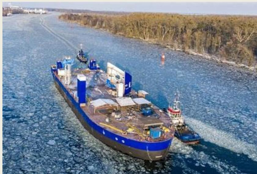
Marine commenced construction of the vessel in March 2025. UAE's Subsea Cable Assets (SCA) has been appointed to deliver the full design, manufacturing, delivery, and commissioning of a cable installation deck spread for the CLV. The newbuild DP2 vessel will be dual-fuel (methanol) prepared, equipped with a 25-tonne offshore knuckle boom crane, a mooring system and will be able to accommodate
