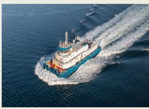
Uzmar Shipyard has completed two pusher tugs for Hidrovias do Brasil and they left the Turkish builder's facilities 17 January 2023 on a heavy-lift vessel. Both HB Mapara and HB Dourada were built to Robert Allan Ltd RApide 4600 design and have dieselelectric propulsion, with three Wärtsilä main engines driving three
