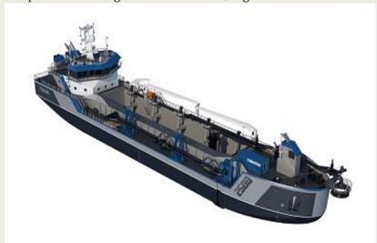
Veritas and Lloyds Register. In close collaboration with Finnish software developer NAPA and Bureau Veritas, Damen has presented the three dimensional design of their TSHD 2500 (Trailing Hopper Suction Dredger with 2500 m<sup>3</sup> hopper capacity). All the mission equipment as specified for a client had been integrated into design. Bureau Veritas this assessed the steel hull structure to be strong enough and safe to
