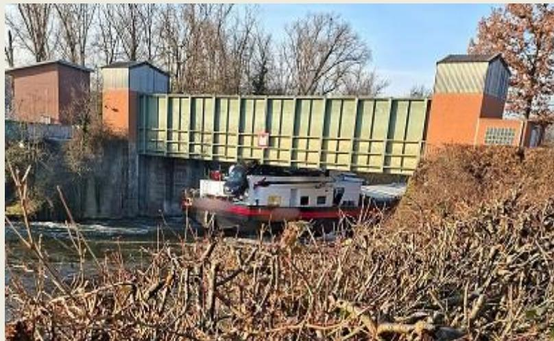
The vehicle had been secured on aft deck which sat too high and
