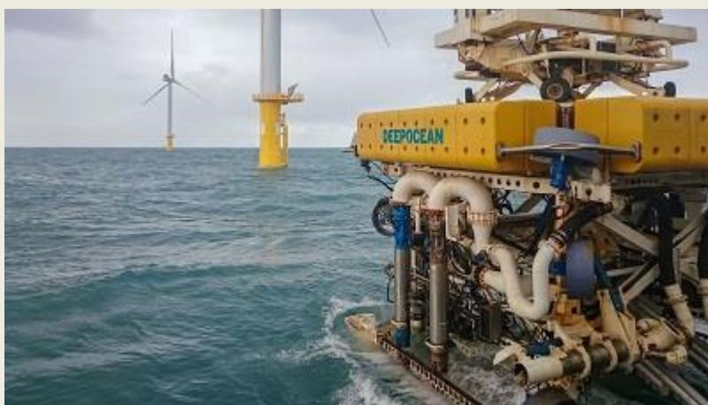
Global ocean services provider DeepOcean has successfully completed trenching and survey operations on inter-array cables for a U.S. offshore wind project. DeepOcean's scope of work encompassed trenching and surveying of the inter-array cables that connect turbines to the offshore substations. These critical operations ensure the long-term protection and stability of the subsea cable infrastructure.
