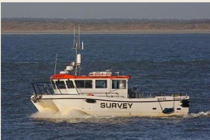
The 10-meter survey vessel **Deep Nordic**, operated by Amsterdam-based Deep Hydrography & Geophysics, has been spotted several times recently in both the Wadden Sea and the North Sea. This catamaran is a Cougar 10M type and was built in Kent, England, by Audacious Marine of Ramsgate. Its shallow draft makes it ideal for seabed surveys in waters close to shore. (*Source: www.maritiemdenhelder.eu; Photo: Frits Alderink*)
