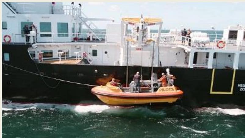
davit systems safely and smoothly handle a maximum weight from 4.5t (S) to 25t (XL) in sea conditions up to a significant wave height of 3.5m (and up to 4.0m in emergency situations). Each system is equipped with a wave compensation system to extend workability and ensure operational safety. An improved cable spooling setup is part of
