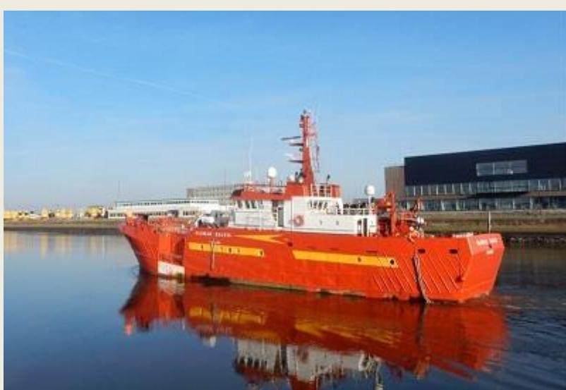
The **Glomar Baltic** standby vessel, towed to Den Helder last week by the **Glomar Linde** due to propulsion problems, returned to sea on Saturday, January 17, after being repaired. Its destination is the Noble Resolute oil rig, which is working at the L10M platform northwest of Den Helder in the Dutch sector of the North Sea. *(Source: www.maritiemdenhelder.eu; Photo: Wim Albers)*
