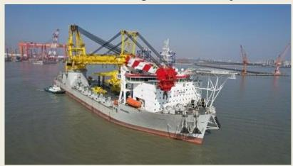
foundations, is now the largest heavy lift vessel in Jan De Nul's fleet. The vessel is capable of installing XXL offshore wind components in floating conditions and with ultra-low emissions, according to the company. The vessel sports a main crane of 5,000 tons, a deck loading capacity of 61,000 tons and a deck space of 9,300 m², enabling it to easily transport several heavier future
