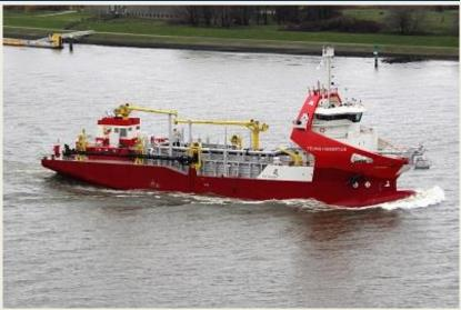
hopper dredger from the series of 'standard' medium-sized hoppers from IHC Dredging – equipped with the latest innovations. The dredger has an optimized hull shape for the lowest resistance possible and is also equipped with a well-balanced efficient engine room. This combination results in best-in-class fuel efficiency with adequate low greenhouse gas emissions, said Royal IHC. (Source: Dredging Today; Photo: Reinier van de Wetering)
