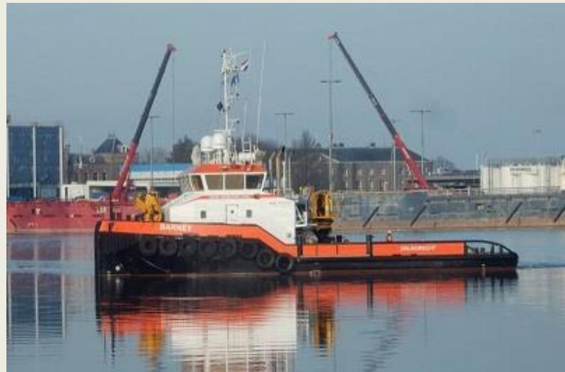
Caterpillar C18 main engines, each driving a propeller in a nozzle. The tug's bollard pull is 30 tons, and its working deck has a surface area of 150 square meters. On Sunday, the Barney departed again to retrieve a lidar buoy in the North Sea. (*Source: www.maritiemdenhelder.eu; Photo: Wim Albers*)
