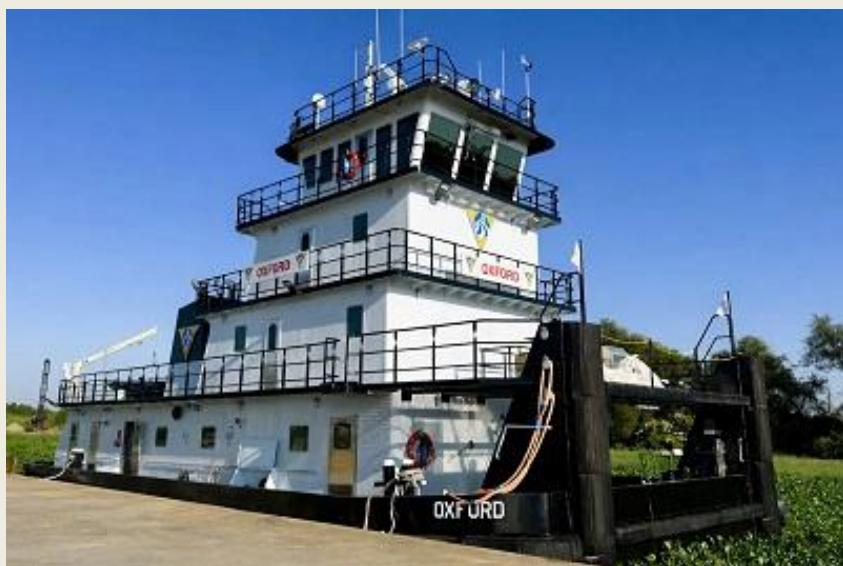
by Intracoastal Iron Works, Bourg, La. A triple-screw 2,400 hp. towboat with four decks, the **Oxford** measures 78 by 34 by 10 feet with a draft of 7 foot, 9 inches. The **Oxford** is powered by three Mitsubishi S6R2 Tier 3 diesel engines from Laborde. The engines turn 72- by 64-inch Hung Shen props on 7-inch shafts with Wartsila seals and Thordon bearings. Reduction is 5.381:1 via Reintjes gears. The boat can carry 28,000
