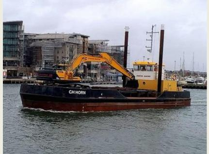
moving vessel the HX Series applies boom floating control, allowing consistently stable operating – perfect for dredging operations. *(Source: Dredging Today)*
