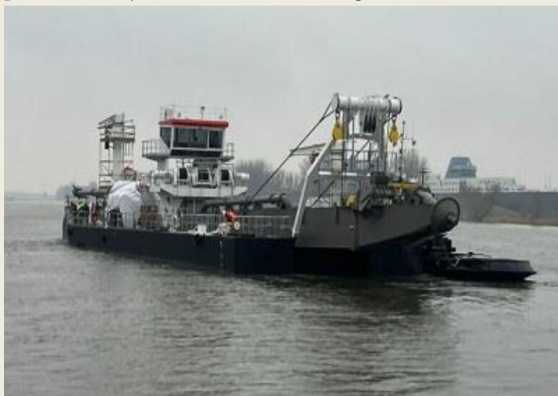
Cutterspecial® pumps in series to reduce wear and enhance operational efficiency, and a powerful cutterhead engineered to cut through cemented silica sand up to 25m depth. Also, the dredger is demountable and road-transportable – essential for deployment to Quarzwerke's silica sands operation in Poland. "We're now moving into commissioning and finalization, after which the vessel will be transported to Poland – ready to
