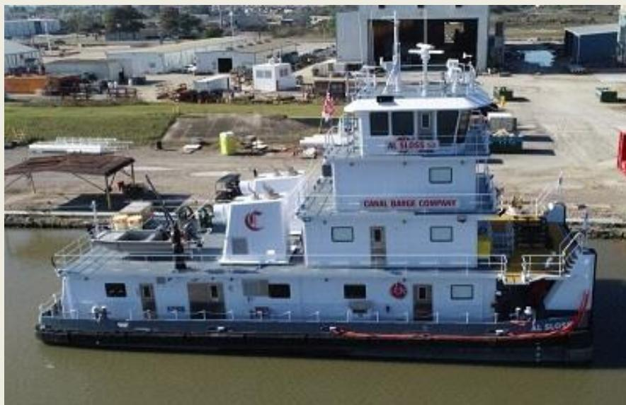
Shipbuilder C&C Marine and Repair, Belle Chasse, La., has delivered the towboat **Al Sloss** to Canal Barge Co., New Orleans, completing the first vessel in a four-boat newbuild series under construction for the operator. The 2,600-hp towboat measures 87'x34' and was designed by C&C's in-house engineering team. Construction was completed on an
