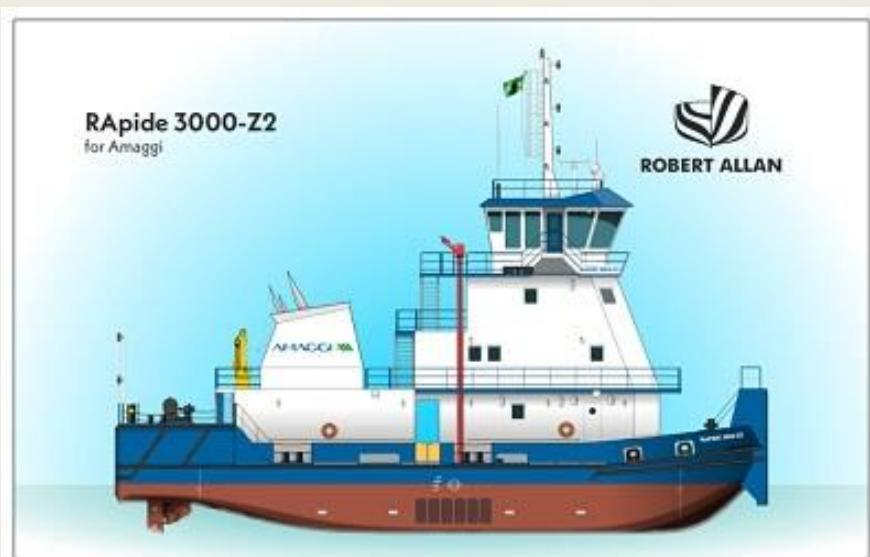
capable of operation with either B100 biodiesel or marine diesel oil. The Z-drives are fully withdrawable afloat and feature 1800 mm fixed pitch propellers for optimal maneuverability and efficiency in shallow water. Electrical power is supplied by two MWM diesel generator sets, ensuring redundancy and reliable operation for all onboard systems. (PR=Robert Allan)
