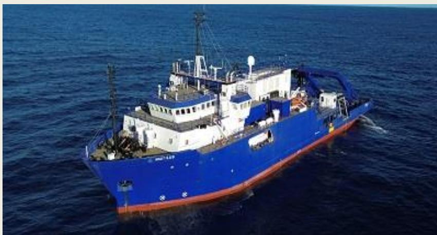
The 75-meter-long DP-II vessel **Nautilus**, which joined TDI-Brooks' fleet in the summer of 2023, is headed to Namibia for a deepwater "heavy" geotechnical project where it will use the jumbo piston cores (JPC) and CPT Stinger geotechnical tools, followed by a second shallow water deep push CPT (Manta-200) project. These projects
