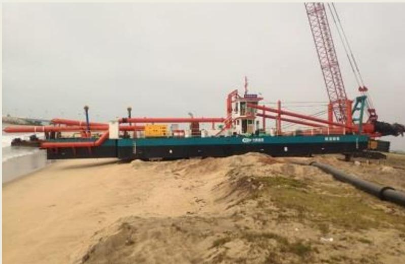
Shandong Haohai Dredging Equipment Co. Ltd (HID Dredging) delivered its **HID CSD500** model cutter suction dredger (CSD) to China Harbor Group recently. According to HID, this piece of equipment comes with a full dredge package, including a 2000m discharge pipes, spare parts, and crew training. The cutter suction dredger 500 (20 inch) is a dismountable dredger with an integrated dredge pump and
