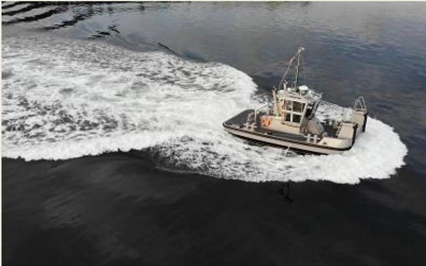
W340 gears, twin Cummins QSL9-SW engines generate 286 bhp at 1,800 rpm each, offering 16,000 lbs of bollard thrust (in forward). The workboats assist barges, submarines, and other naval vessels; open and close security barriers; and tow and push floating port operation support equipment. Additional shipyard projects underway at Snow & Co. included a
