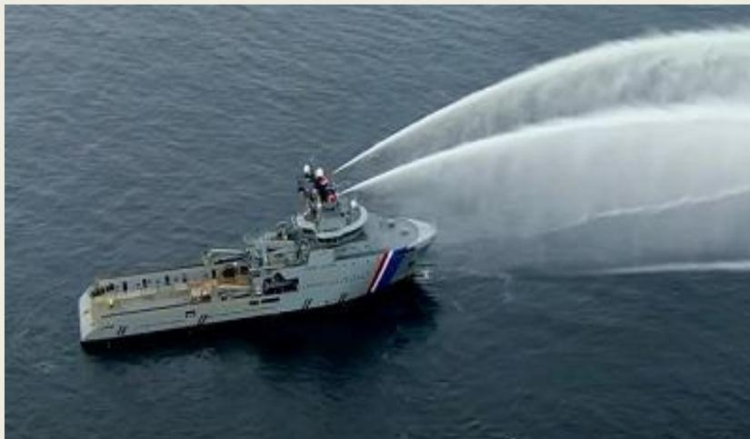
The patrol ship **Freyja** has proven itself particularly well in the more than three years it has been in the Icelandic Coast Guard fleet. The ship is well equipped and includes powerful fire extinguishers that are extremely efficient. They can pump about 7200 cubic meters of water per hour and throw the water about 220 meters from the ship. This equipment needs to be tested
