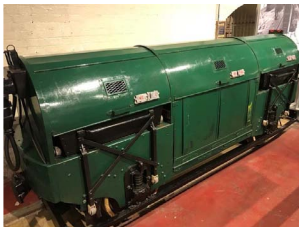
An original fully automated driverless '90 English Electric' locomotive as used in 1927 (Picture: David Kerridge)
