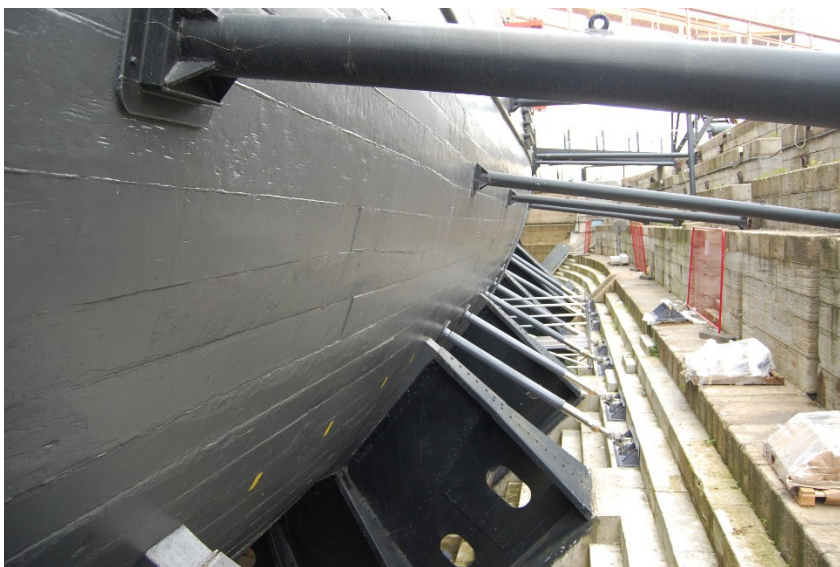
Original hydraulic supports in position in 2017
