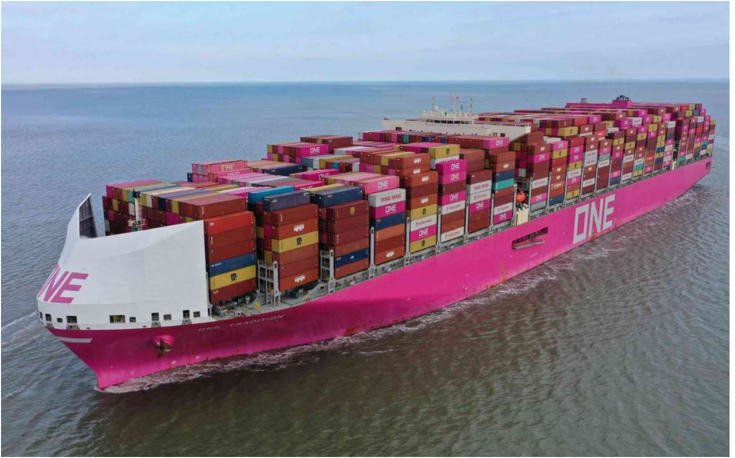
Two superb views as she enters the harbour, the wind shield was fitted in March 2023 to improve aerodynamics and save fuel. “One Tradition” is capable of 21,700 TEU and is just a few centimetres under 400 metres long. (Photos contributed)
