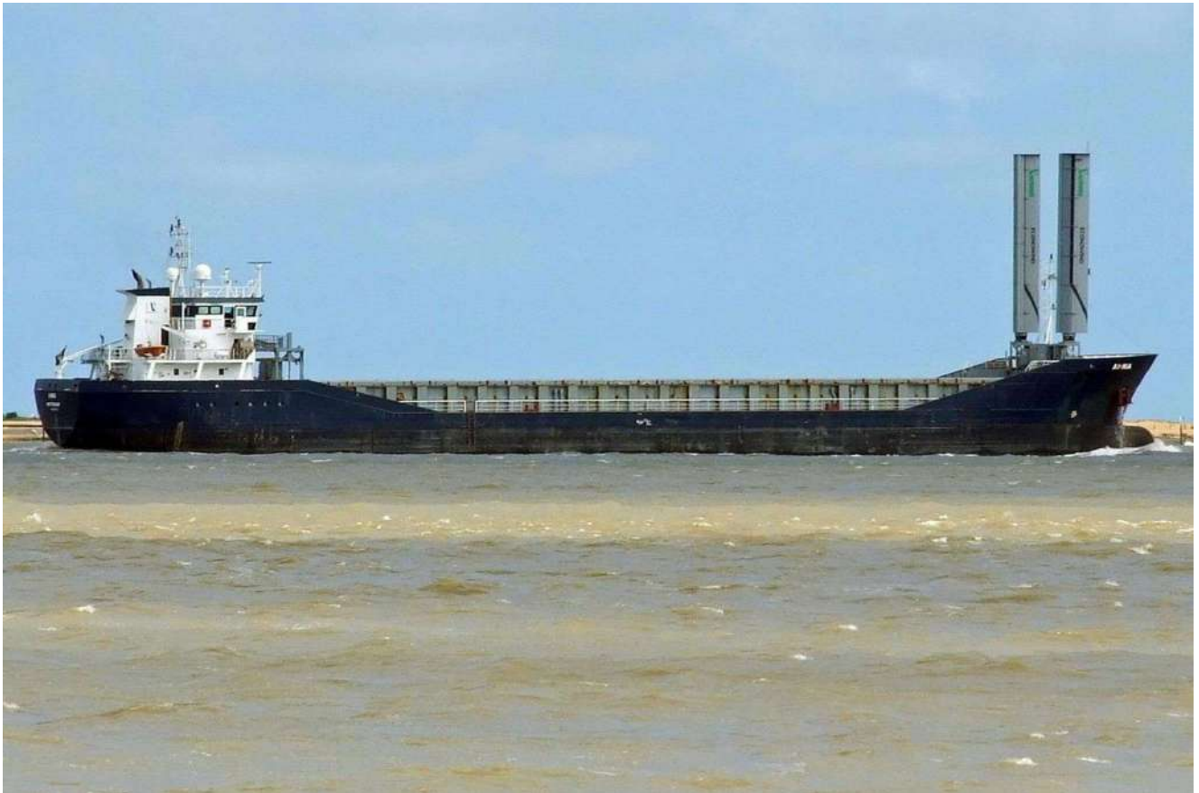
Spotted with her Econowind Ventfoils installed mid 2022, “Anna” outbound from Ipswich for Schiedam on 6 th June. Her owners Vertom have signed a contract for retrofitting several of their ships with Ventfoils. Built in 2008 by Barkmeijer, Stroobos as “Blue Sea” she became “Beaumerit” in 2011 and her current name in 2016. During all these changes she remained under the Dutch flag. (Photo by Mick Marshall)
