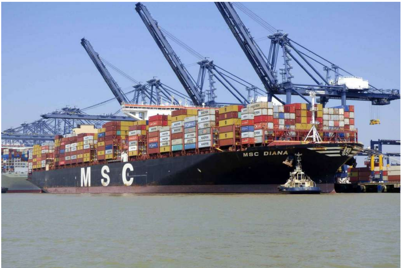
Getting ready to sail for Tanger Med from number nine berth on 10 th June is “MSC Diana” . She had arrived at Felixstowe from Antwerp on 7 th June. Built by South Korean yard, Samusng, Koje in 2016 she is 399.9 metres long and 58.8 beam. The 19,462 TEU vessel was recently fitted with an exhaust scrubber. (Photo by Mick Warrick)
