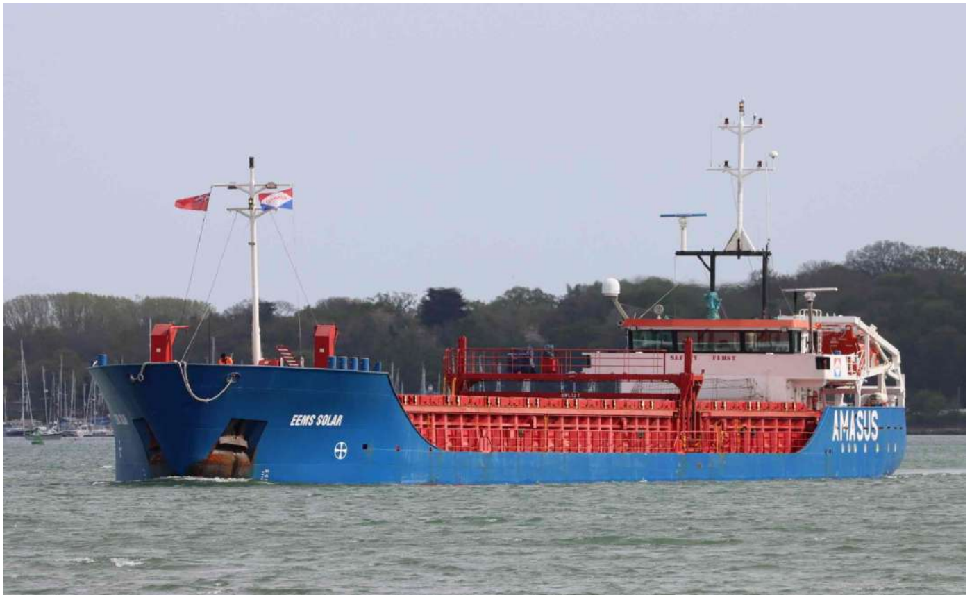
Nearly at voyage's end as "Eems Solar" approaches the port of Ipswich on 16 th April. She has come from the French port of Nantes which counts sand amongst its exports. Built in Vietnam at Haiphong by 1-89 Enterprise shipyard in 2010, she was one of six ships of this class later lengthened in the Ukraine. She sailed for the Cork anchorage on the 17 th and laid there until the 22 nd when she set off for the Waalhaven, Rotterdam. (Photo by David Hazell)
